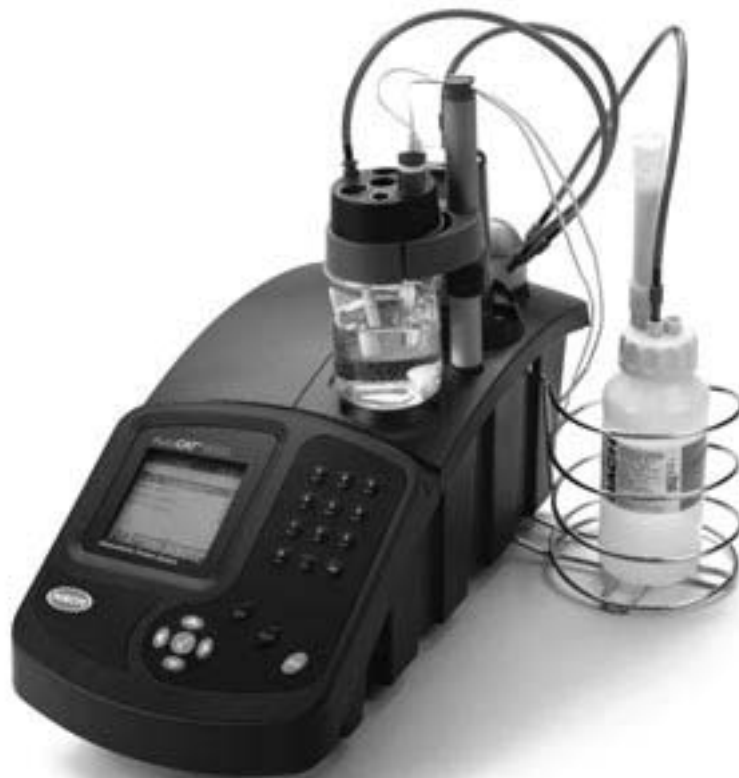
Figure 2.4: Hach Company’s AutoCAT 9000 Amperometric Titrator
